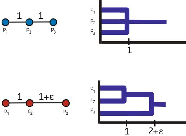
**Fig. 5.** Complete Linkage is not stable to small perturbations in the metric. On the left we show two metric spaces that are metrically very similar. To the right of each of them we show their CL dendrogram outputs. Regardless of  $\epsilon > 0$ , the two outputs are always very dissimilar.
